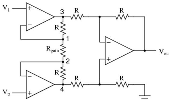
**Figure 11.1** Block diagram of Instrumentation amplifiers
