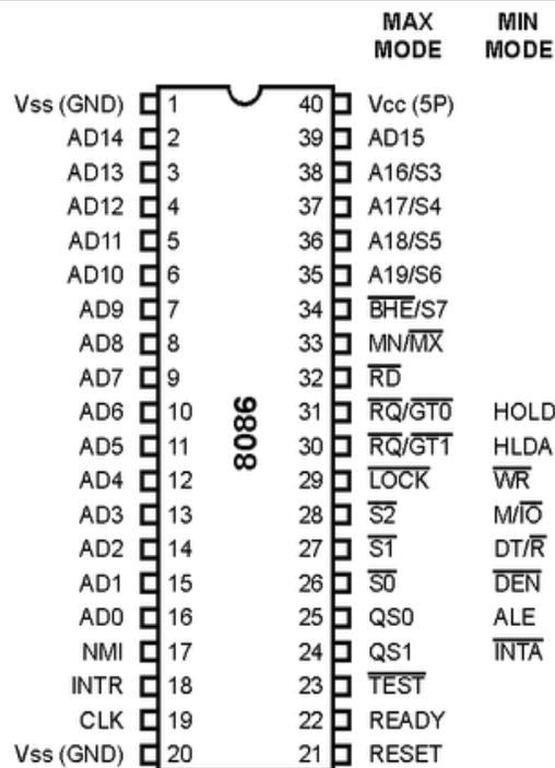
Figure 2.2 Pin diagram of 8086
