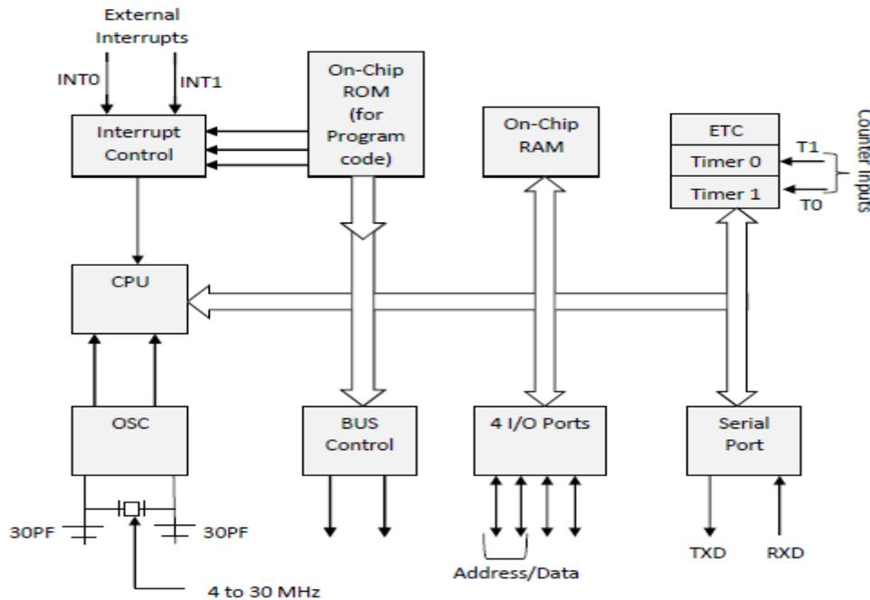
**Figure 5.1 Block Diagram of 8051 Microcontroller**
