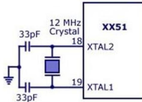
**Figure 5.5 8051 clock circuit**
