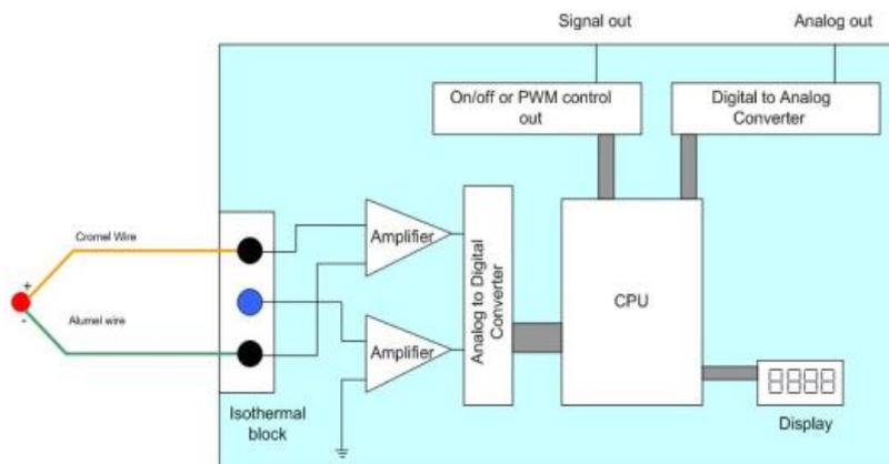
**Figure 10.2** Scheme for temperature monitoring and controlling
