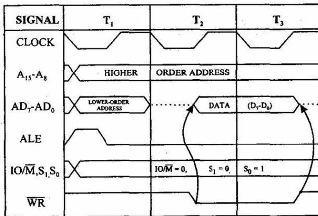
Figure 1.4 Timing Diagram for Memory Write cycle
