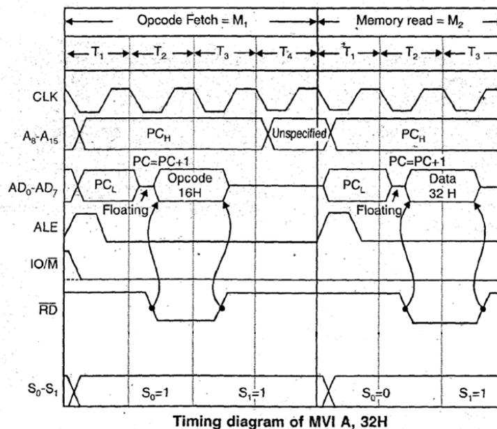
**Figure 1.3 Timing Diagram for Memory Read**
