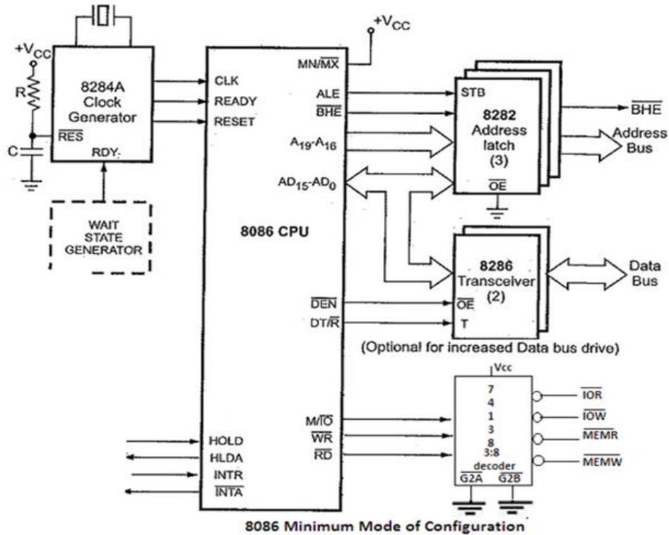
**Figure 2.5** Minimum mode functions of 8086
