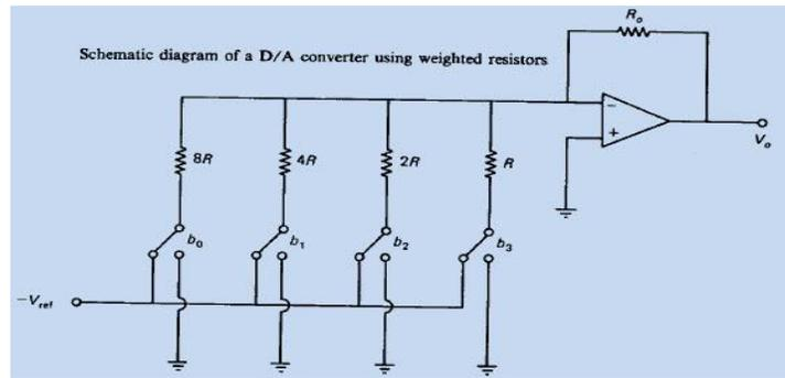
In the voltage domain, that is if the input signals are voltages, the addition of the binary bits can be achieved using the inverting summing amplifier shown in the above figure.
