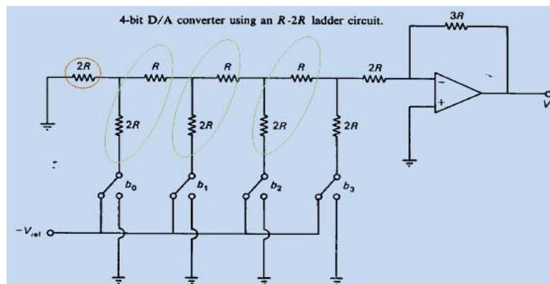
The above figure shows the 4-bit R-2R ladder DAC. In order to achieve high-level accuracy, we have chosen the resistor values as  $R$  and  $2R$ . Let the binary value  $B_3 B_2 B_1 B_0$ , if  $b_3=1, b_2=b_1=b_0=0$ , then the circuit is shown in the figure below it is a simplified form of the above DAC circuit. The output voltage is  $V_0=3R(i_3/2)= V_{ref}/2$
