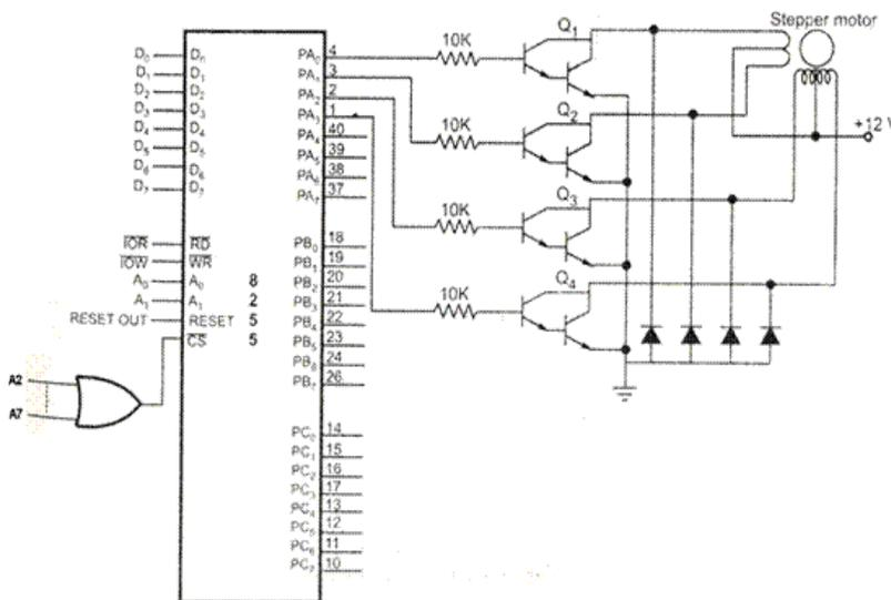
**Figure 10.4 Interfacing stepper motor with 8085**
