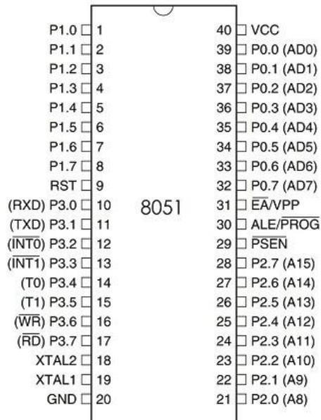
**Figure 5.2 Pin diagram of 8051 microcontroller**
