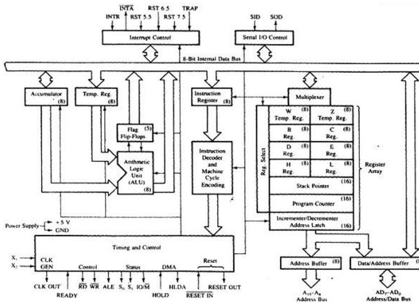
Figure 1.1 Architecture of Intel 8085
