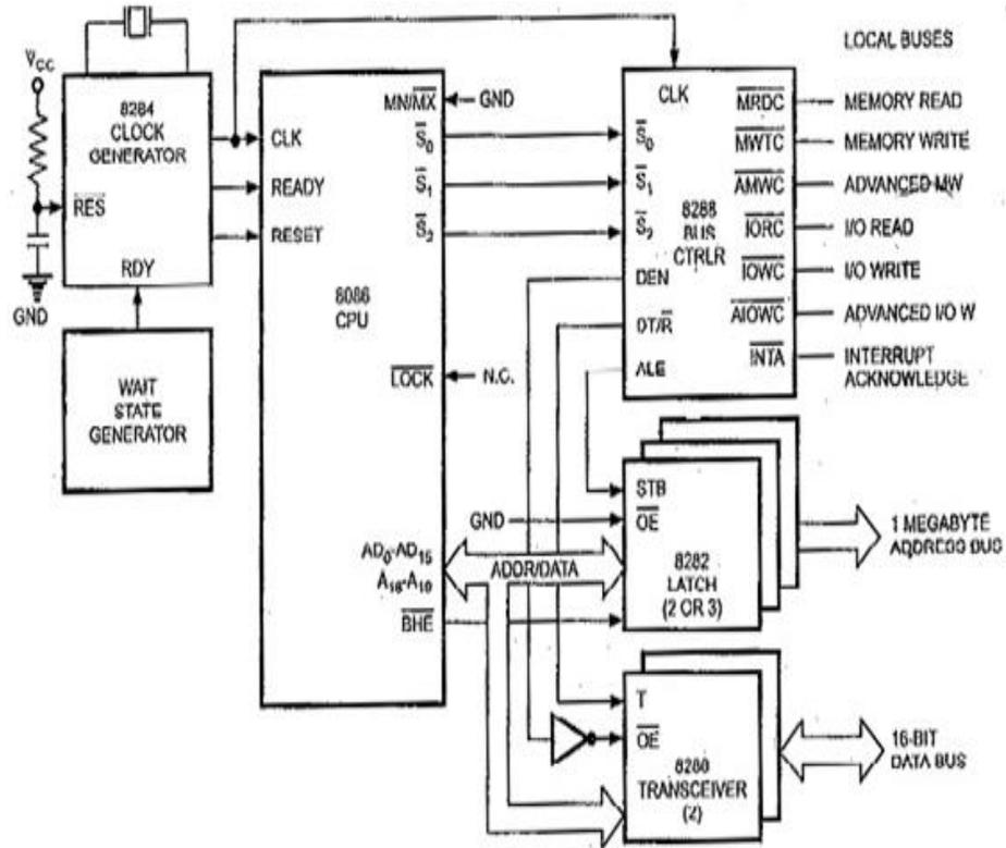
Figure 2.4 Maximum mode functions of 8086
