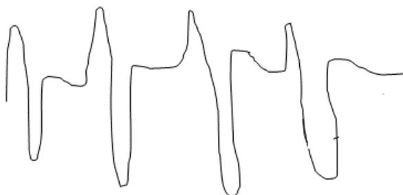
Fig.13.3 ESR spectrum of methyl radical  $^{120}\text{CH}_3$
