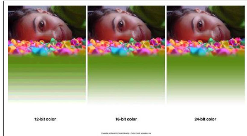
Figure 3-21 An example of different levels of posterization that can occur across multiple device color depths
