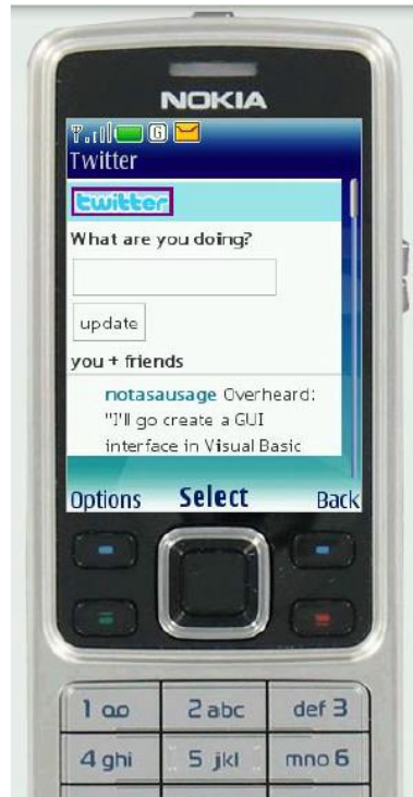
Figure 3-20 Example layout of a scroll-based application where the user had to press the D-pad past each link to scroll the page
