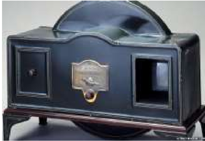
Fig. 9.1 The Baird 'Televisor': The First Commercial Television Set to Receive the 30-line Pictures (1929-1935)
